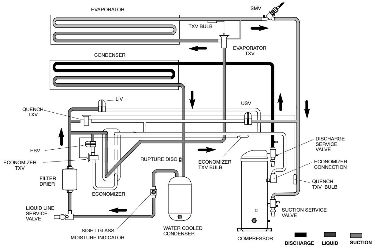
Figure 2-7 Refrigeration Circuit Schematic - Standard Operation
