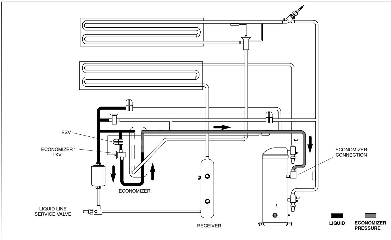
**Figure 2-8 Refrigeration Circuit Schematic - Economized Operation**
