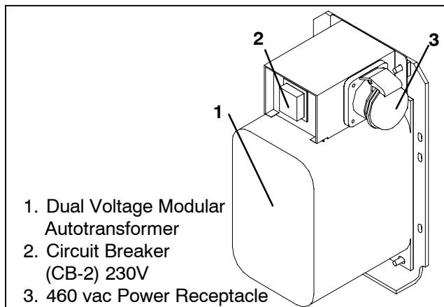
Figure 4-1 Autotransformer
