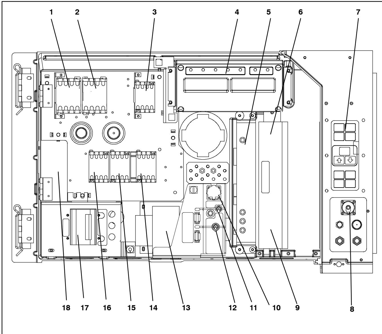
1. Compressor Phase A Contactor
