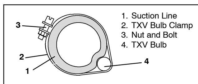
**Figure 6-10 Thermostatic Expansion Valve Bulb**
